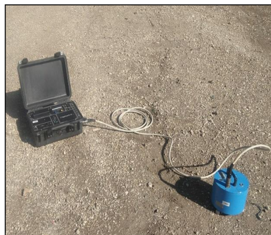
Figure 2. Equipment used for ambient recording (CityShark II station Lennartz-5 s sensor)
